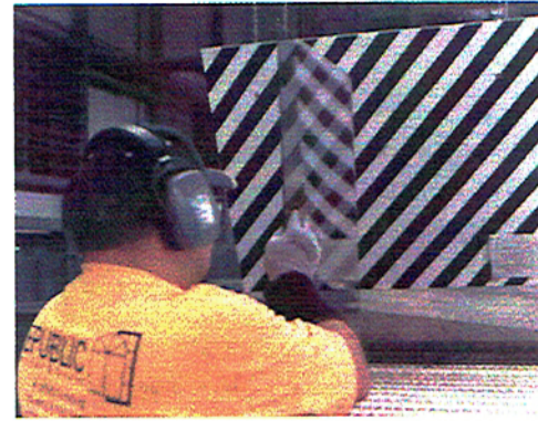
An operator checks a piece of finished T.U.F.® glass for waviness and quality as it comes out of Republic's in-house tempering oven. Republic tempers hundreds of pieces of glass per day.
