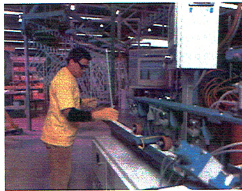
Republic was one of the first vinyl window manufacturers to incorporate Super G Warm-Edge technology into all of its window lines. Here, an operator assembles a tin-plated u-shaped steel spacer, the integral component in Republic's Super G™, warm-edge insulated glass.
